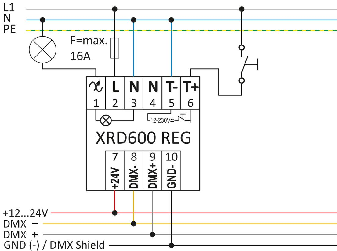
Fig. 2 - Connection diagram with push button 230 VAC
