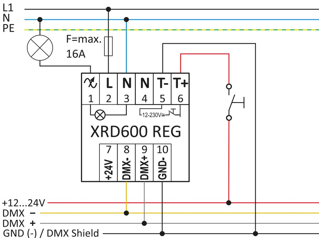
Fig. 3 - Connection diagram with push button 24 VDC
