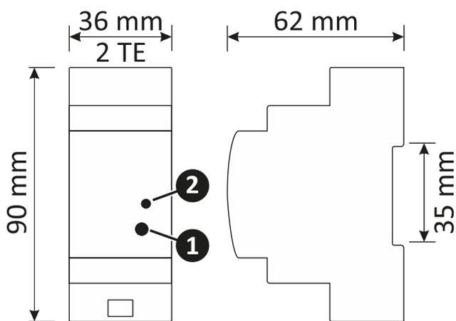
Fig. 1 - Housing dimensions and connections
