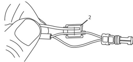
Insert each the red+ with the red wire and the black with the red / black wire between the sheath and the connectors (1) and press down with your hand the blade connectors (2) firmly.
