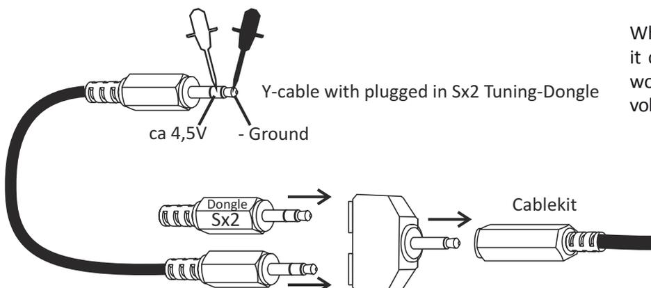
When it is plugged in with a Y-adaptor it can also be checked if the dongle is working. With an inserted dongle, the voltage is reduced to approximately 4.5 V.
