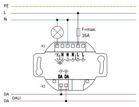
Fig. 3 - Connection diagram with DALI
