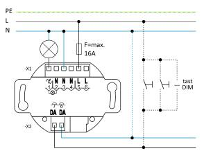
Fig. 4 - Connection diagram with 230 VAC push button (tastDIM)
