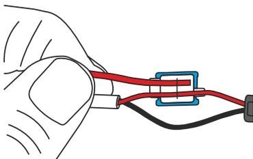
The related wires of the speedsensor and the wire / wires for the power (as shown in the manual for the cablekit) are inserted into the through-opening of the blade connectors. Now press down with your hand the blade connectors firmly.
